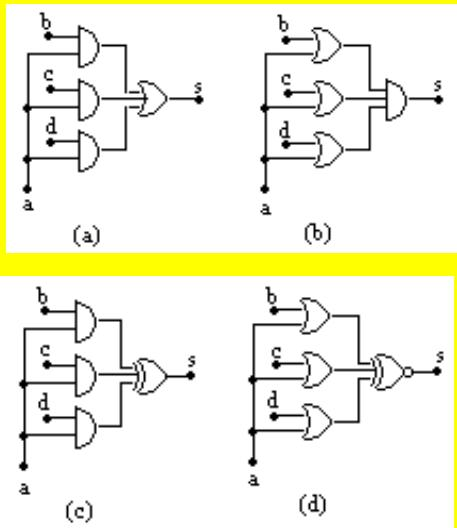
$$\begin{aligned} (a) \rightarrow s &= ab + ac + ad = a(b + c + d) \quad \text{dist.} \cdot \% + \\ (b) \rightarrow s &= (a + b)(a + c)(a + d) = a + bcd \quad \text{dist.} + \% \cdot \\ (c) \rightarrow s &= ab \oplus ac \oplus ad = a(b \oplus c \oplus d) \quad \text{dist.} \cdot \% \oplus \\ (d) \rightarrow s &= (a + b) \otimes (a + c) \otimes (a + d) \\ &= a + (b \otimes c \otimes d) \quad \text{dist.} + \% \otimes. \end{aligned}$$
