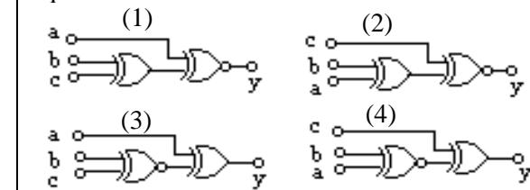
$$\begin{aligned} (1) \Leftrightarrow y &= a \otimes (b \oplus c) = a(b\bar{c} + \bar{b}c) + \bar{a}(bc + \bar{b}\bar{c}) \\ &= c(ab + \bar{a}b) + \bar{c}(ab + \bar{a}\bar{b}) = c \otimes (b \oplus a) \Leftrightarrow (2) \\ &= a(bc + \bar{b}\bar{c}) + \bar{a}(bc + \bar{b}\bar{c}) = a \oplus (b \otimes c) \Leftrightarrow (3) \\ &= c(ab + \bar{a}b) + \bar{c}(ab + \bar{a}\bar{b}) = c \oplus (b \otimes a) \Leftrightarrow (4). \end{aligned}$$
